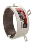
B1 Fire Collar is designed to maintain the fire resistance of fire rated walls and floors where these are breached by continuous plastic pipes, for use in gypsum, masonry and concrete walls and floors. The steel shell contains a graphite based reactive material which reacts when exposed to heat, closing the openings left by the softening plastic pipe.
